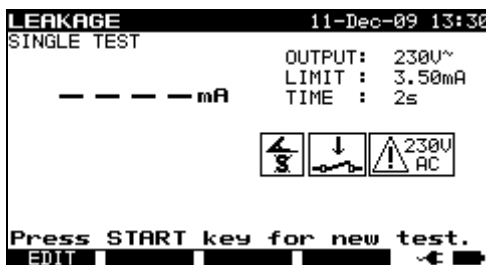
Differential leakage current menu
