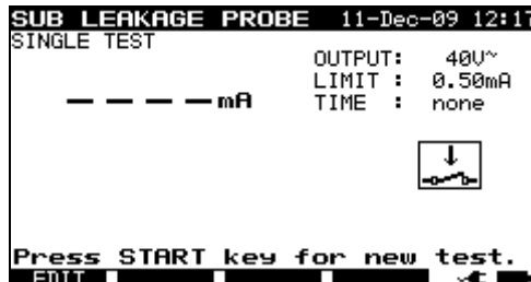
Sub leakage – S probe menu
