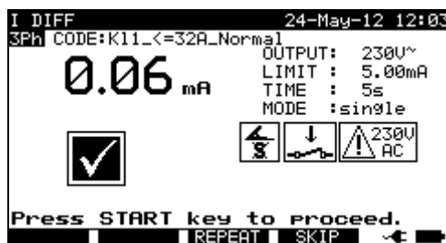
Primary leakage current autotest menu
